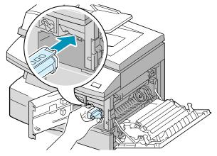
**5** Reinstall the toner cartridge, and then lock the lever.
